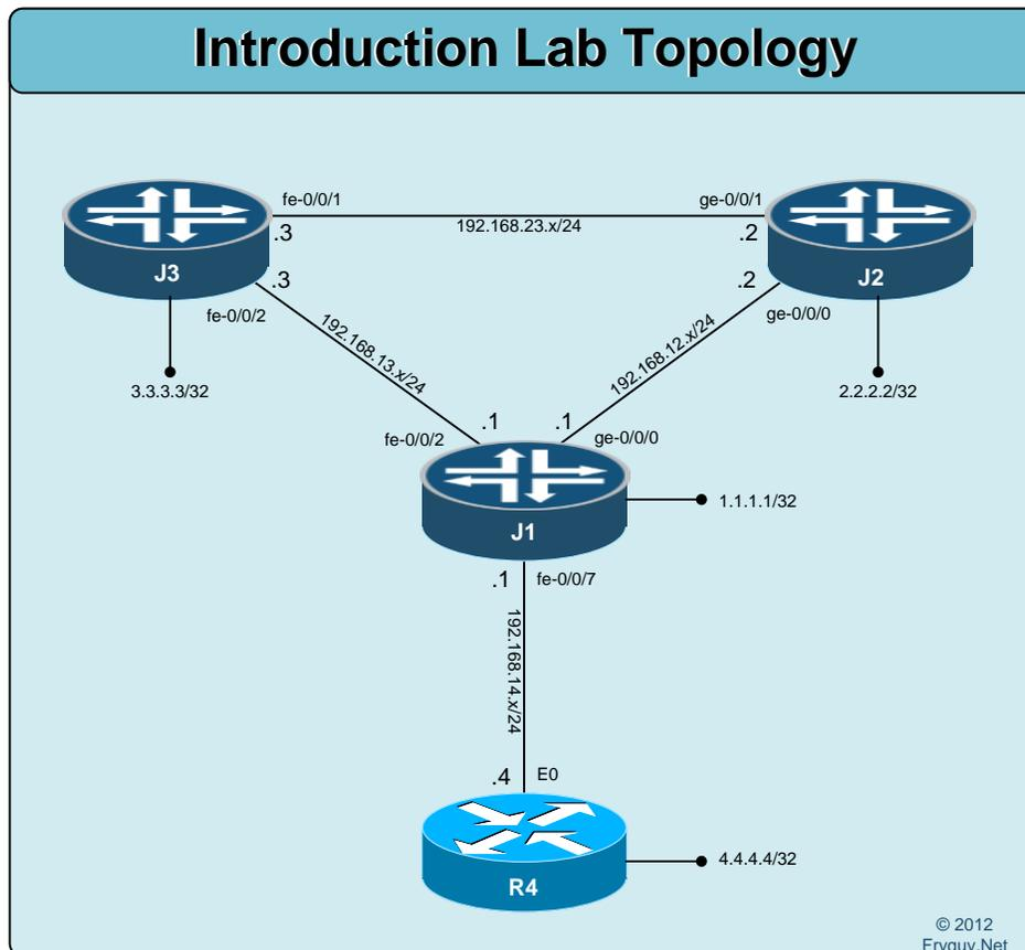
Now it is time to get some housekeeping done on these routers. We will configure the interfaces on each of them. Once that is complete, we will create a Rescue configuration. A rescue configuration is a known working configuration that we can roll back to at any time. We will use this rescue config to reset the routers to a base state before each lab.
