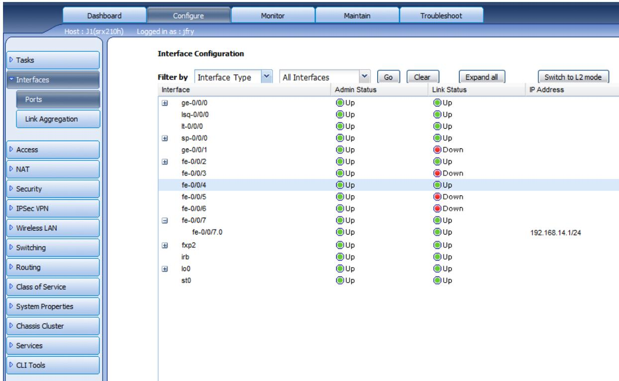
If we look at the monitor tab and select the interface (here fe-0/0/7) that connects us to R4, we can see we have some traffic being generated. ( I set off a bunch of 9000 byte pings )
