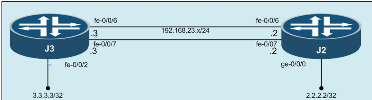
Once that is cabled, we can now configure our LAG connection between the two devices.
