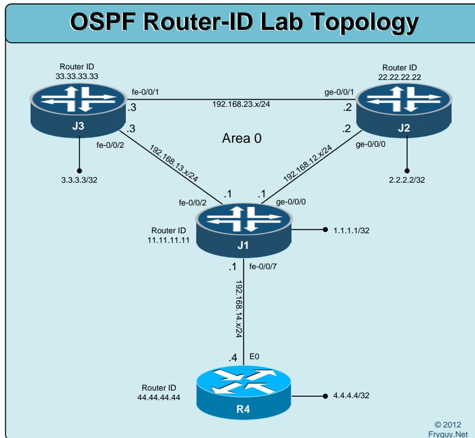
Ok, time for some of the other things that we might do with OSPF. First up, router-ids. For this lab, we will create router-ids in the form of xx.xx.xx.xx where x=Router number. For example, R4 will be 44.44.44.44, and we won't use a loopback interface for this.
