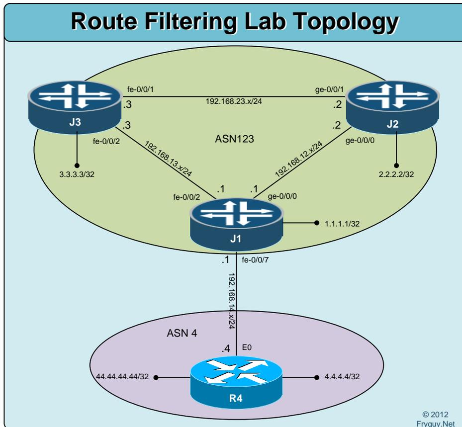
Ok, let's discuss Route Filtering in this lab, and to keep it simple, we will use eBGP for the routing protocol. For this lab we will need to create another loopback on R4 for 44.44.44.44/32.
