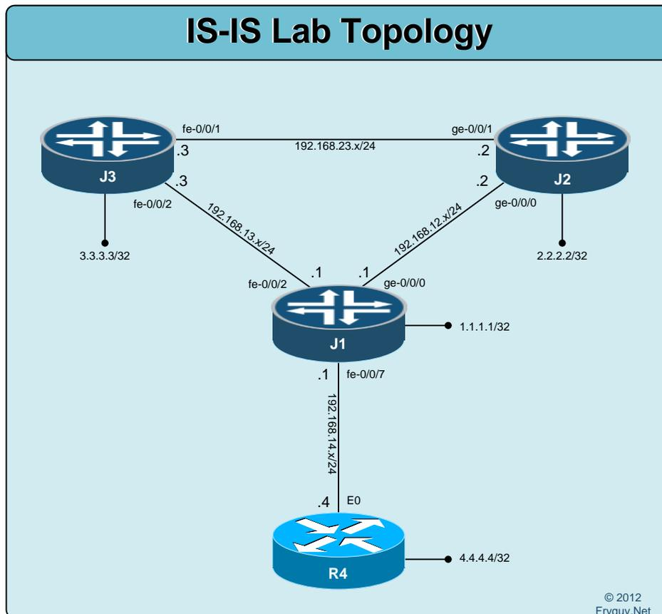
Time to do some IS-IS labs. I am going to try and make these short and simple. I am sure as I get more into Junos I will write more complex IS-IS topologies and start to include LDP as well.
